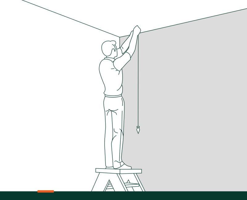
Hang the first strip using a plumb line to get a perfect vertical. Hang the subsequent strips relative to the first strip, matching pattern as required
